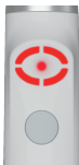
Battery power is too low 4 segments flashes rolling and displayed as red
